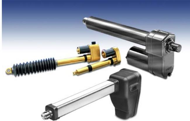
Electric actuators replace hydraulic cylinders in mobile off-highway vehicles to eliminate troublesome fluid leaks and make the vehicles smaller, lighter, and quieter.
