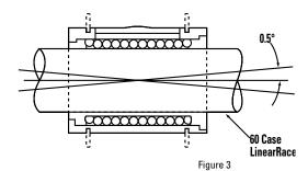
Super Ball Bushing Bearing Self-Alignment Feature
