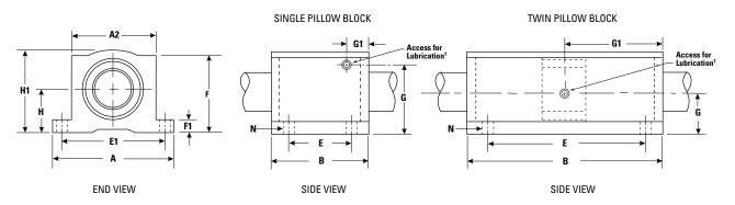
† Sizes .25, .375 and .500 have oil lubricant fitting. Sizes .625 and above have 1/4-28 access for lubrication.
