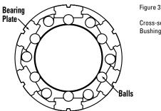
Cross-section of Super Ball Bushing Bearing
