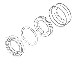
Lube for Life modification kits provide continuous bearing lubrication and enhanced protection for a broad range of applications. The Lube for Life attachments consist of a section of oil-saturated polymer actively compressed by a contact spring, inside a standard pillow block seal. Mod Kits are for use with non self-lubricating Super and Super Smart Ball Bushing® Bearing pillow blocks. Each Mod Kit includes two Lube for Life cartridges and assembly instructions.
