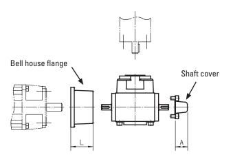
To be able to install the gear to the motor a bell house flange must be used between the gear and the motor. The bell house flange, which includes a matching coupling, is ordered separately. A shaft cover can be ordered to cover the second primary shaft on the gear in case it is not being used.
