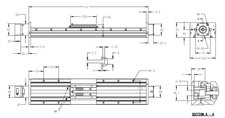
A1: lubrication nipples (using the unit with the nipples mounted makes the stroke 10 mm shorter).
