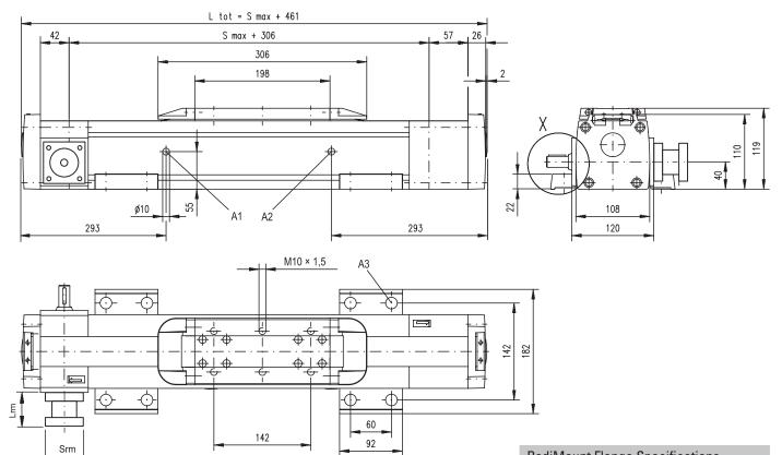
A1: lubrication hole A2: lubrication hole (no hole if L order is < 856 mm) A3: ø17/ø10,5 for socket head cap screw M10
