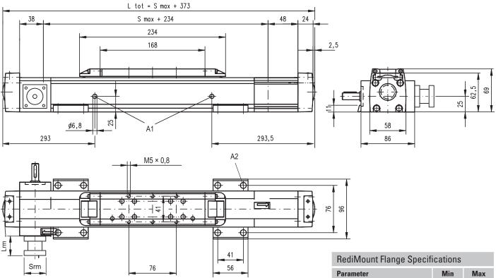
A1: lubrication holes A2: ø9,5/ø5,5 for socket head cap screw M5
