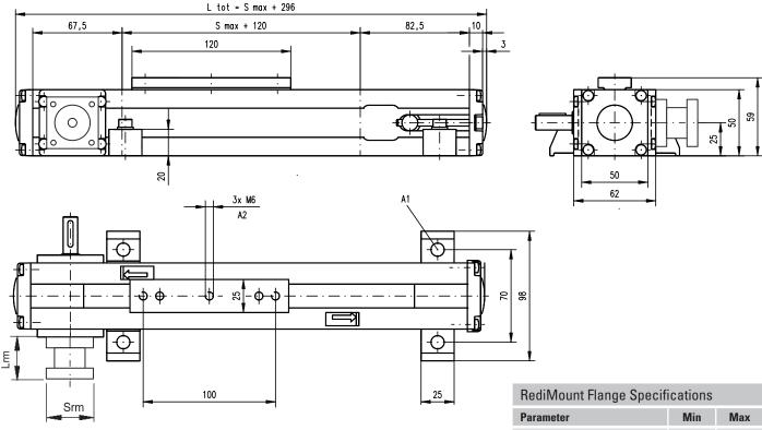
A1: ø6,5 for M6 screw A2: depth 9, Heli coil
