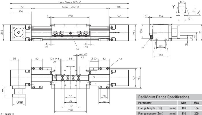
A2: funnel type lubricating nipple DIN3405-M6×1-D1
