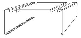
The protective shrouds are made of metal and protect the drive mechanism of the unit from dust and dirt but leave the guides unprotected. Shrouds do not reduce the stroke of the unit but they will add 4 mm to the width of the unit. Shrouds are ordered mounted from factory and are stated in the ordering key of the unit.
