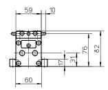
A1: depth 11 A2: socket cap screw ISO4762-M6×20 8.8
