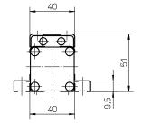
A1: depth 10 A2: lubricating nipple on both sides DIN3405 D 1/A
