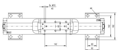
A1: slide guide tensioning holes ø6 (MG10N), ø10 (MF10N) A2: 127,5 if Ltot <=1055mm, 227,5 if Ltot > 1055mm (MG10N), 292,5 (MF10N) A3: 34,5 (MG10N), 56,5 (MF10N)
