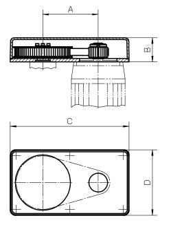
BGM belt gears can only be used on units without a RediMount flange. The belt gear comes in parts and is assembled to the unit and motor by the customer.
