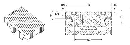
Bellows protect the unit from dirt and dust. Note that the bellows option reduces the available stroke of the unit by 28%. Bellows can be ordered and mounted at the factory - see ordering key. Bellows can also be ordered separately and fitted by the customer. In that case, order two pieces of bellows where the length of each bellows piece = stroke length of the unit × 0.86.
