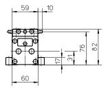
A1: depth 11 A2: socket cap screw ISO4762-M6×20 8.8 A3: tapered lubricating nipple to DIN71412 AM6 A4: can be changed over to one of the three alternative lubricating points by the customer
