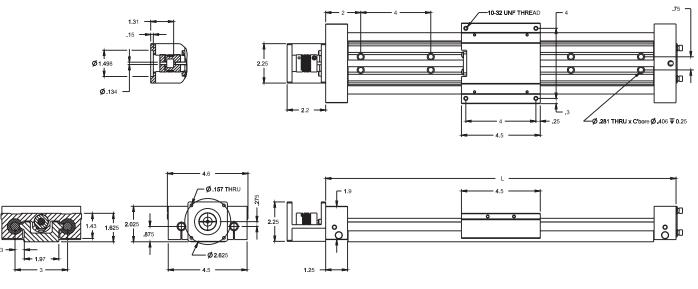
Standard NEMA23 motor dimensions are shown. Other mounting sizes are available and easily configured. Please see www.LinearMotioneering.com for details.
