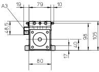
Parameter Min Max Flange length (Lrm) [mm] 83 145 Flange square (Srm) [mm] 90 200 Flange weight \* 5,64 [kg]
