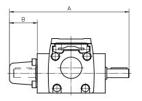
The shaft protection cover is used to cover shafts which are not being used. The covers are fitted by the customer.
