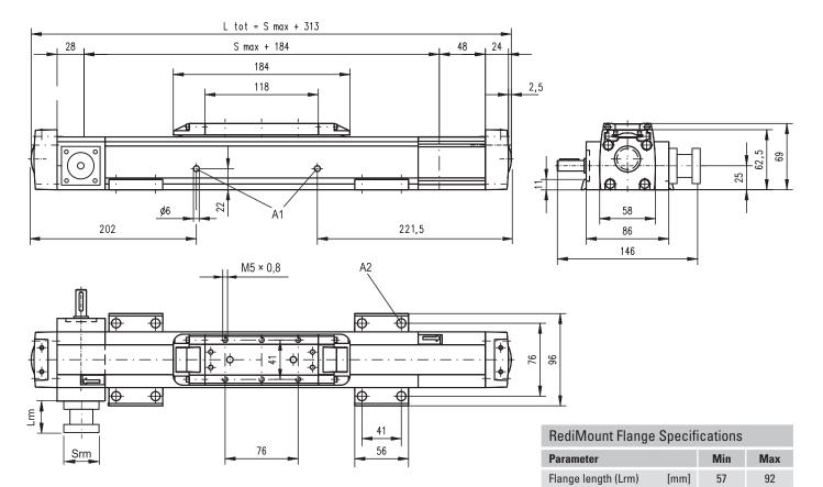
A1: slide guide tensioning holes A2: ø9,5/ø5,5 for socket head cap screw M5
