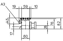
RediMount Flange SpecificationsParameterMinMaxFlange length (Lrm)[mm]83145Flange square (Srm)[mm]90200Flange weight \*[kg]5,64
