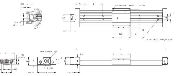
Standard NEMA23 motor dimensions are shown. Other mounting sizes are available and easily configured. Please see www.LinearMotioneering.com for details.
