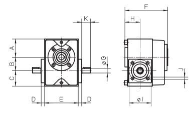
The worm gear is installed directly to the unit and requires no intermediate coupling between the two.
